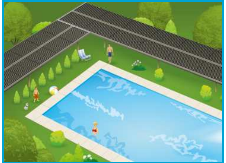
Turbosorber Large system also acts as a pergola - provides pleasant partial shading. - can also be supplied with supports for snow loads.
